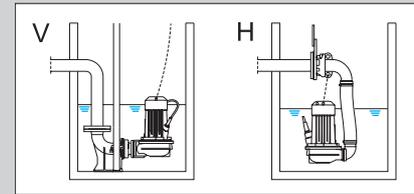
Pumps are available for permanent fixed installation, using the guide rail coupling V or the header coupling HK, that is installed above the water level.
