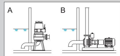
Pumps with cooling system can be used in permanent dry flood-proof immersible installation A. For conventional dry installation B refer to the BW series brochure.
