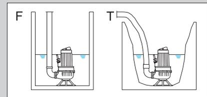
All pumps can be delivered for semi permanent free-standing installation F with stand and discharge adapter or for transportable use T with non-overloading impeller.
